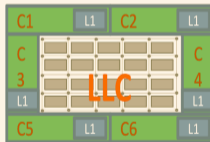
A Chipmultiprocessor (CMP) with non-tiled architecture.
